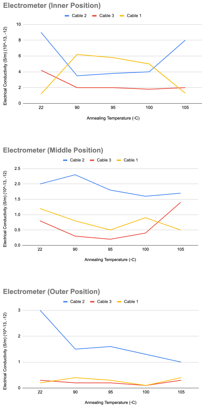
Figure 3. This figure displays the electrical conductivity that resulted from the annealing temperatures at different positions. The yellow line demonstrates cable 1(XLPE-15), the blue line represents cable 2(XLPE-0), and the red line represents cable 3(XLPE-30)(Xie et al., 2020).
